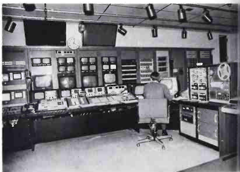
Operator in front of keyboard unit of CDL's APC 610-200 in master control which can interface with business automation systems. FCC log printer to far right.
