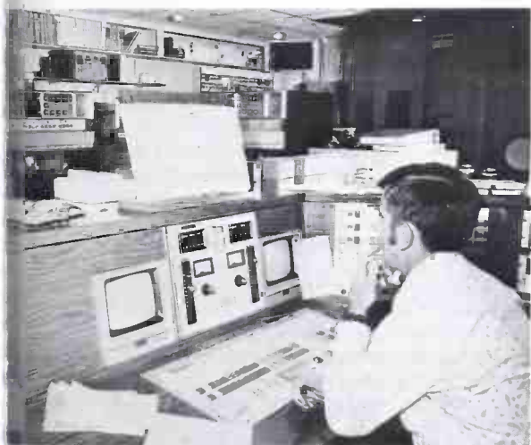
Operator at WTOG sits at Sarkes-Tarzian video production computer, which provides basic control of programming. Unit is a modification of APT-2000, adapted to specific needs of station, which has extremely busy scheduling.
