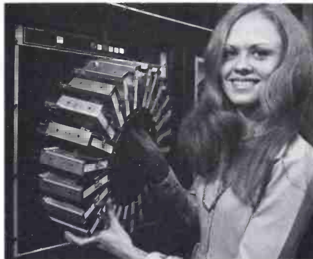
Control Design Corp.'s CD24R Multiple Cartridge Machine with unique removable drum; holds 24 standard cartridges, access time 6 secs.
